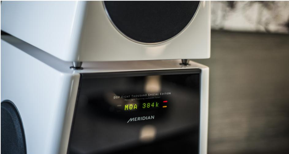
*From the very beginning, Meridian loudspeakers have been Active – including the amplifiers and line-level crossovers inside the cabinet. But Meridian had taken the leap into digital audio technology with the introduction of the Compact Disc several years earlier: it had been evident to Meridian's founders that an all-digital signal path from the source to the loudspeaker was the future.*
